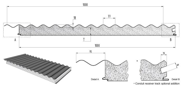
Insulated Corro-EPS-FR is an Insulated Roof Panel System, comprising of two pre-painted, roll-formed steel skins, with a fire retardant grade expanded polystyrene insulating core.
